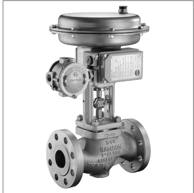
Fig. 5: Control valve with integral attachment of a digital Ex 'd' positioner designed to be connected to Ex 'd' systems
